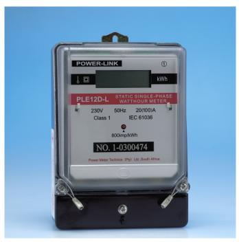
High metering security against illegal abstraction and fraud is one of the main features of the PLE12D-L. Protection from mechanical, magnetic, or electrical interference is built into the product by careful circuit design and layout. As an anti-fraud feature, the meter runs forward regardless of the energy direction. The meter will thus register correctly even if it is reverse connected, making it the ideal choice for metering end consumers in the modern energy market.
